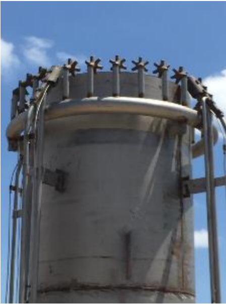
This is a close-up of a refinery flare tip. The pronged ends are used to insert steam during flare events.
