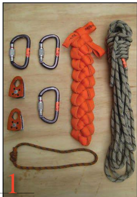
Figure 1. Equipment needed to build a piggybacked 4:1 haul system.
