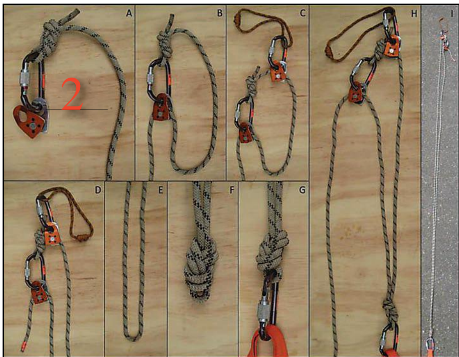
Figure 2. A) Sequence of steps used to build an optimized 4:1 haul system. A) Install a pulley at the rope terminus, B) Clip a bight of rope in the pulley, C) Install a second pulley in the loop created, D) Extend haul system to lip edge or until the rope nearly pulls through the haul system, E) Tension both sides of the rope and find the bight closest to the anchor, F) Tie a knot in the bight, G) Clip knot to the anchor, H) Full 4:1 haul system extended to the lip, I) Haul system extended to the full length of the rope.
